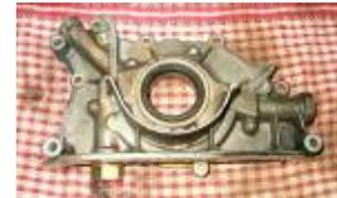
Ensure you use **lock tight** on the bolts when assembling the oil pump as they are known to rattle loose causing a gradual loss of oil pressure.
